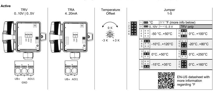
fig. (Measuring range and offset adjustment, default settings: 0 °C..+100 °C | 0 K)
